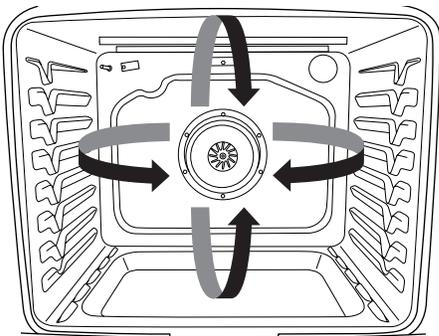
During convection baking or roasting, the bake, broil, and convection elements cycle on and off in intervals while the fan circulates the hot air. During convection broiling, the broil and convection elements cycle on and off.
