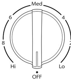
The control knobs can be set to anywhere between HI and LO. Push in and turn to setting.
